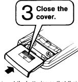
Be sure that you insert the batteries so that their positive (+) and negative (-) polarities match the polarities indicated in the compartment. Batteries installed with incorrect polarities may leak and damage.
